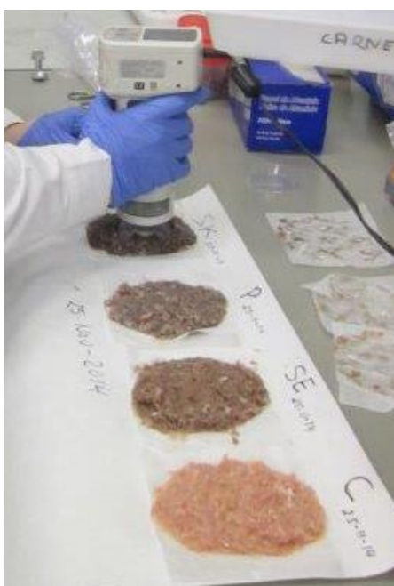
Figure 6.34. CIE-LAB color measurement with a CR-400 Chroma Meter
