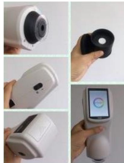
Figure 4.2. CIE LAB color measuring instrument spectrophotometer
