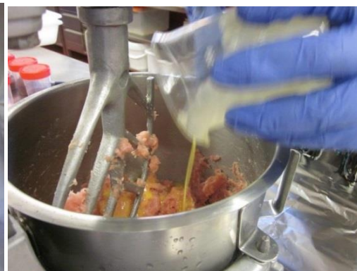
Figure 6.18. Blending of minced meat in a bowl mixer with the other ingredients
